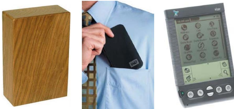
**FIGURE 6.6** Before starting development of the early Palm Pilot, inventor Jeff Hawkins carried a block of wood, the size of the potential Pilot, in his pocket for a week to explore how the idea felt.
